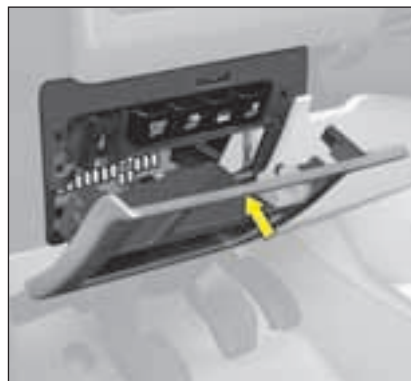
Access to the first fusebox under the dashboard
